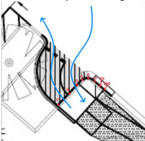
The grades at the wing should help the cyclist on the inside curve i.e. City-bound, which is good. (I've shown paths as if they're following the nominal edge of path.) However, the travel path for the other direction is still a bit tight.
