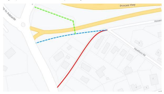
Other implications are shown in <u>Sheet 4</u> in particular: the path/s provided cannot be maintained at 3.0m in width, with a 1.8m path used to access Waverley Court off Waverley Ridge Road. (See <u>Sheet 4</u> comments). This is a significant constraint in terms of the quality of the facility provided, especially coming on top of constraints imposed by the bridge crossing of the Princes Highway.
