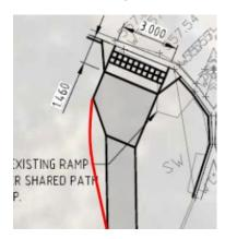
e) Path width, eastern side – Rather than transitioning to the existing path width (apparently 1.2m), we suggest widening this section of path as much as possible, noting that the continuation on Sheet 2 is 1.5m wide. While 1.5m is narrow for shared use, this is acceptable for one-way travel given a bike lane exists on the other side of the kerb, and given that a path separated from the road is necessary to cater for children.
