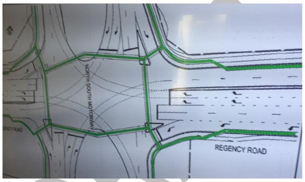
**Example 1:** An alternative design to a stand-up lane: the only access is via the footpath/signals.
